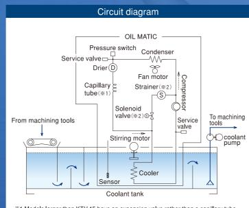
\*\*1 Models larger than KTV-15 have an expansion valve rather than a capillary tube.
